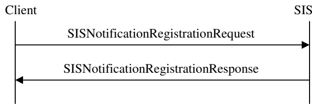
Figure 49: SIS Notification Registration Message Exchange
