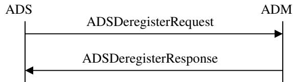
Figure 40: ADS Initiated Deregistration Message Exchange
