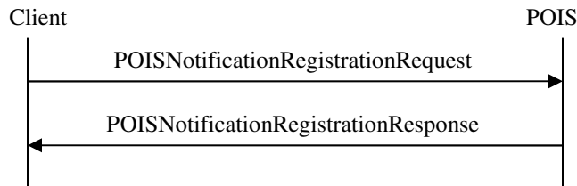
Figure 62: POIS Notification Registration Message Exchange
