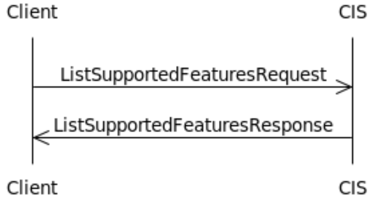
Figure 71: CIS Discovery Sequence Diagram
