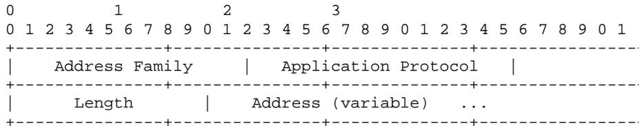
**Figure 6–11 - Route Format for `WithdrawRoutes` and `ReachableRoutes`**
