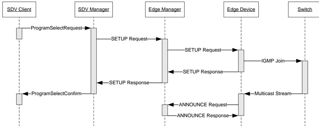
**Figure I-4 - Message Flow for Asynchronous Mode**
