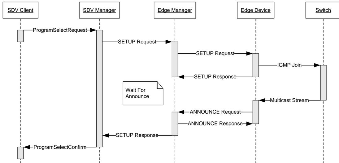
**Figure I-3 - Message Flow for Synchronous Mode**
