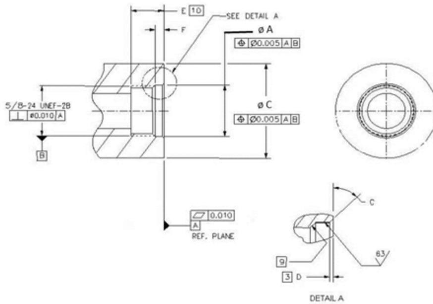
Figure 1 - Physical Dimensions for 5/8-24 Port, Adapter Female
