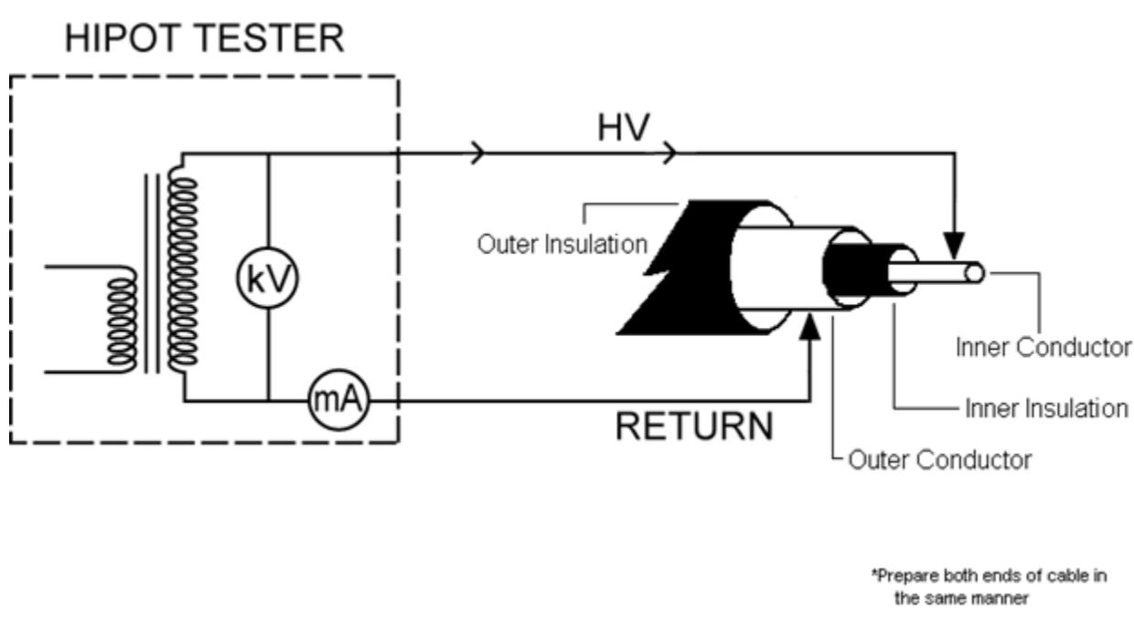
**Figure 2 - Connection Diagram**
